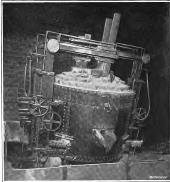
Fig. 7. Booth-Hall Furnace of Four-ton Capacity
